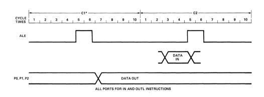
FIGURE 2. 8021 TIMING DIAGRAM
